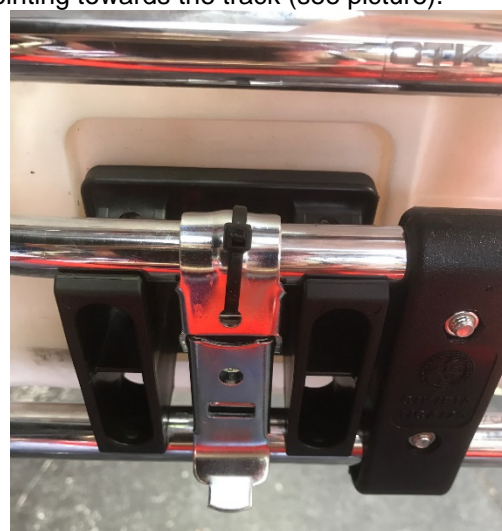
CIK NOSE CONE FIXING METHOD FOR CIK/02.
